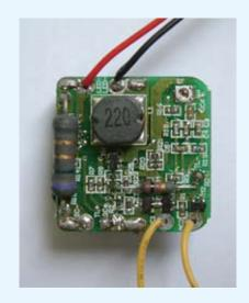
發電花鼓驅動式LED自行車燈整流模組 Hub Dynamo Powered LED Bike Light Rectified Module
