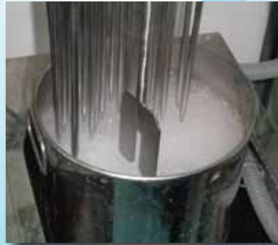
小央廚之高溫急速冷卻機 The usage of cooling machine for small central kitchen
