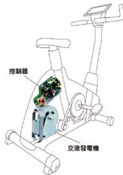
智慧健身發電控制系統 R-Rider (Fitness Equipment Energy Regenerating System)
