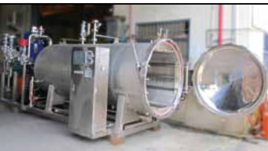
板式熱交換之水淋式殺菌釜 Plate Heat Exchanger for Sprinkle Type Retort
